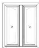
Double shutter inside/outside opening side hung window
